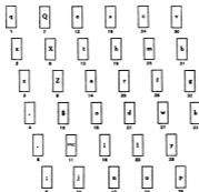
LOWER CASE AND POINTS IN 34-CHANNEL AUXILIARY MAGAZINE (Linotypes with Separate Auxiliary Keyboard)
