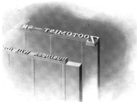
Two-line Initial Matrices cast slugs such as these
