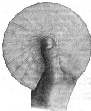
FIGURE 34—Some Monotype rules. This picture shows one minute's product—twenty two-point rules (18 picas long) cut as cast, as clean and as even as a deck of cards. Twenty rules a minute—count 'em
